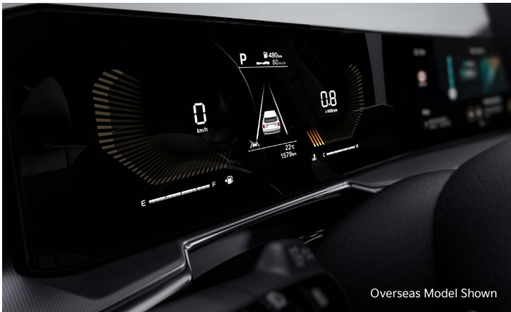
Instrument cluster (4.2" Colour LCD Type: LX+ & Light grades) (12.3" Colour LCD Type: EX, Deluxe, Premium, Earth & Water grades)
